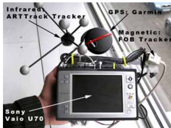
Figure 2: This handheld AR platform is based on a mini tablet PC that is operated as a video-see through “magic lens” device. It currently supports five different tracking technologies (3 shown) and weighs less than 1.5kg.
