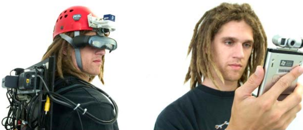
Figure 1: A typical backpack setup (left) for mobile AR and a lightweight handheld device (right).
