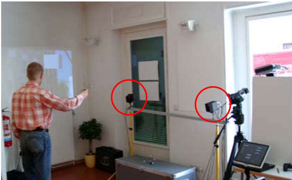
Figure 26: ART tracking system (two camera setup) for precise optical indoor tracking.
