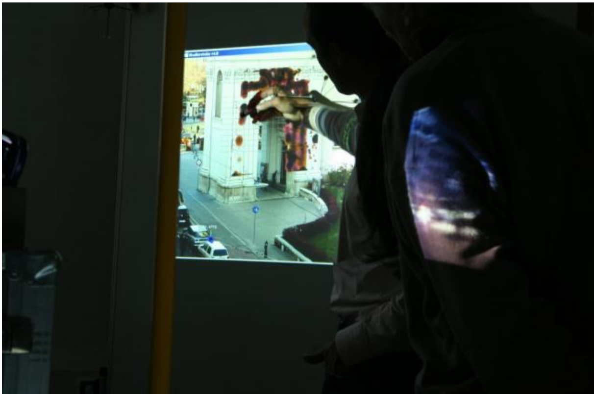
Figure 30: Video see-through augmentation using the camera which delivers live video and with the urban sketcher application.
