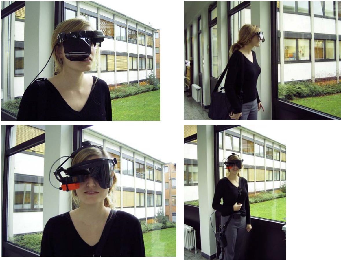
Figure 9: Shimadzu Data Glass 2 (top left) notebook based mobile AR system (top right), Liteye 750 (bottom left), mobile AR system with ultra mobile PC (bottom right)
